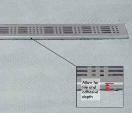
**7** The grate needs to be flush with the tiled surface (tile + adhesive). Raise the whole drainage channel using the 2mm and 4mm selfadhesive spacers.
