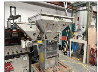
Piovan model MDW 250/41 Gravimetric blender
