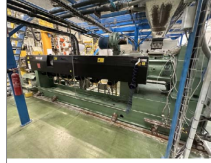
130mm Davis Standard Single Screw Extruder
