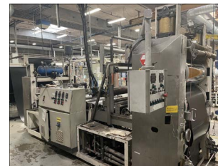
1040mm wide Welex 3 roll polishing stack
