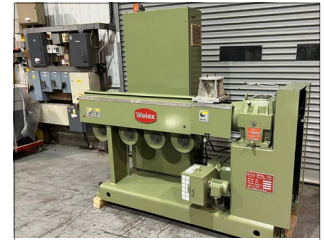
50mm Welex single screw extruder
