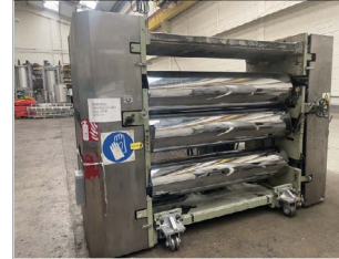
1956mm Welex sheet 3 Roll Stack
