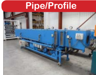
250mm dia Speedex 6m dual vacuum pipe calibration tank
