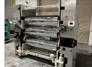
1650mm wide Welex 3 roll polishing stack
