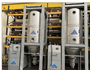
1200 litre hopper with Model D400 Rotordryer
