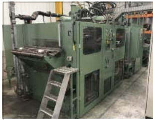
500 x 280mm Illig Model RDM 50K pressure former
