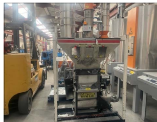
4 Component Maguire model WSB940 blender with hopper
