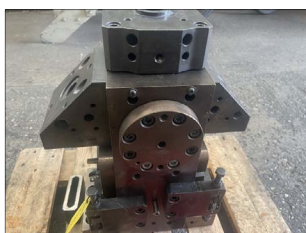
5 layer variable vane Cloeren coextrusion feedblock
