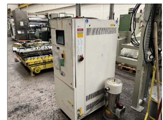
500 Litre Moretto Model 0205 Dehumidifying Dryer
