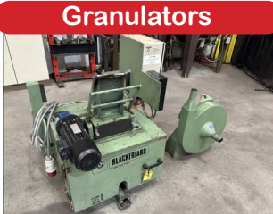
320 x 150mm Blackfriars model 32/15 granulator
