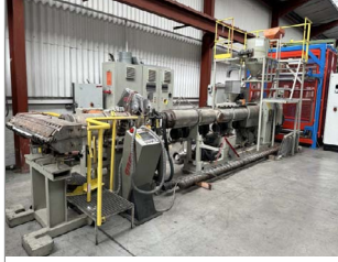
120mm Battenfeld Single Screw Extruder
