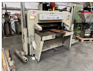
1150mm Wide Polar Guillotine model 115 CE
