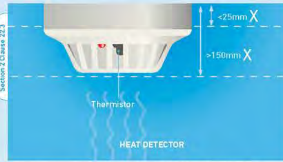
The sensing element of a heat detection device should not be less than 25mm below ceiling, and not greater than 150mm below ceiling.
