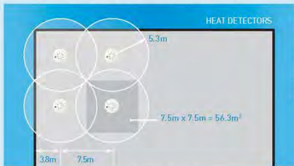
When mounted on a flat ceiling, heat detection devices have an individual coverage of 5.3m radius. However these radii must overlap to ensure there are no 'blind spots'. Therefore individual coverage can be represented by a square measuring 7.5m x 7.5m giving an actual area coverage of 56.3m 2 per device.
