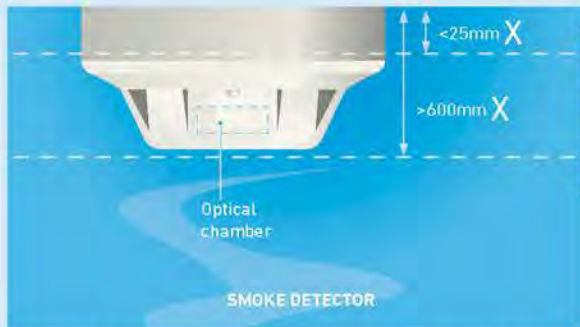
The sensing element of a smoke detection device (optical smoke or ionisation chamber) should not be less than 25mm below ceiling, and not greater than 600mm below ceiling.
