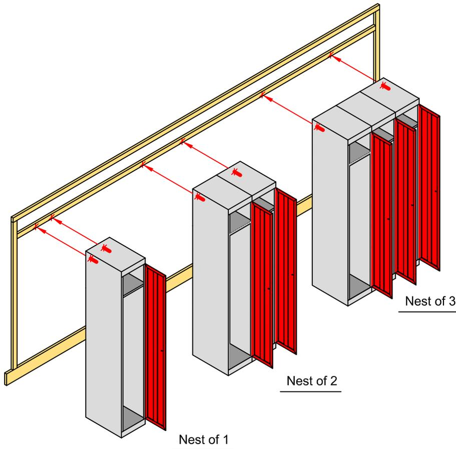
Fix lockers side by side to create runs of lockers using nesting bolts supplied.
