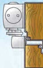
Mounted on the transom of the push side of the door
