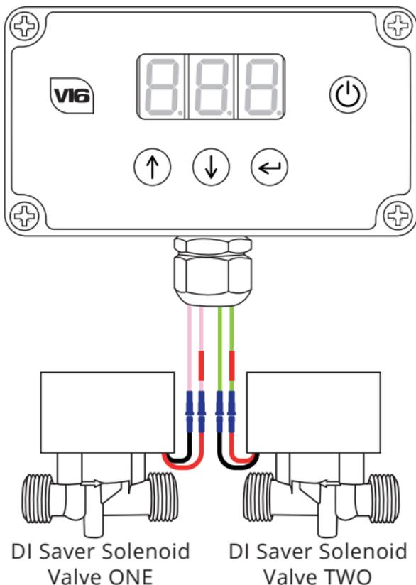
Connect the pump controller in accordance with this diagram.
