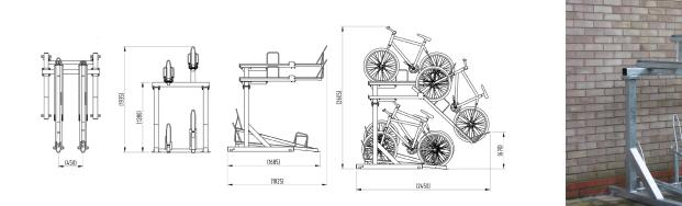
The Double Stack Cycle Rack is designed to maximise the number of bicycles that can be stored in an allotted area. Two wheel grippers at either end of the trough firmly hold the top level bicycle in place.
