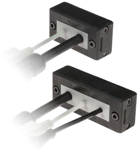
The DES L2 and L3 splittable frames enable pre-terminated cables from 2 to 16mm in diameter to pass through enclosure walls, providing strong strain relief and water protection.
