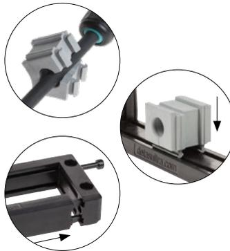
The DES 24 cable entry system consists of a splittable frame designed to accommodate small (SPP), multiple (X) or large (SPG) inserts for cables. The inserts can be freely positioned into the frame.
