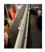
Attach 3 x silver cross bracing to each side using M5 nuts supplied.
