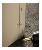
Repeat process for each corner with two screws per corner.
