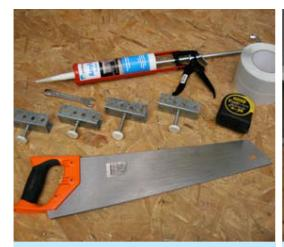
1 Check you have all tools needed. Marmox Bath Panels come in two sheets, 1800mm x 600mm x 30mm and 800mm x 600mm x 30mm.
